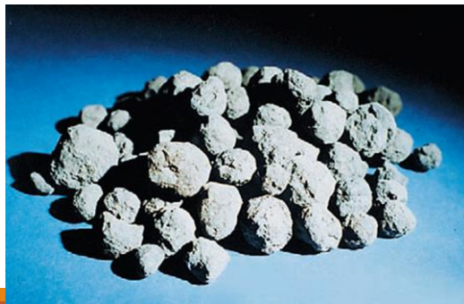
4. Clinker with gypsum is ground into portland cement and shipped.
